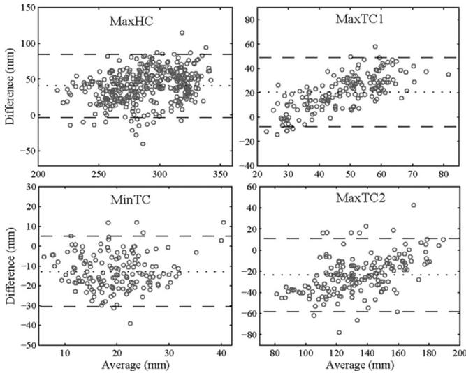
Fig. 3. Bland and Altman plots of the mean (dotted line)  $\pm 1.96$  STD limit of agreement (dashed line) of the difference between the 3-D model with LS approach and reference for foot-clearance parameters.
