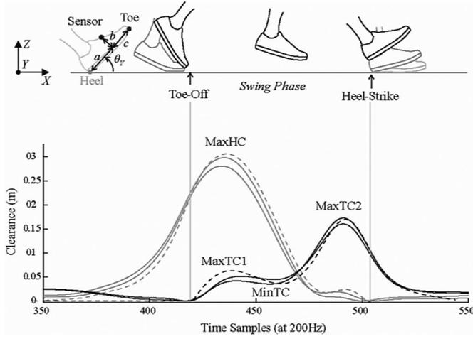
Fig. 2. Sensor location relative to heel and toe  $\{a, b, c\}$ . Schematic of foot kinematics, temporal events, and clearance parameters during one gait cycle. Heel (light gray) and toe (dark gray) clearance are dashed for 3-D model ( $Z^{3D}$ ), and plain lines for internal and external reference markers ( $Z^{REF}$ ).
