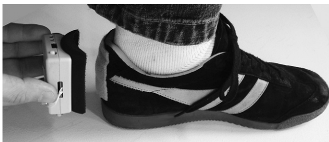
Fig. 1. S-Sense module with compliant foam attached to shoe.
